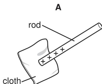
electrons move from the rod onto the cloth
