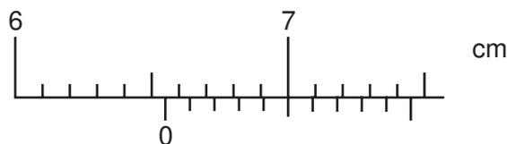
What is the reading on the vernier scale?
