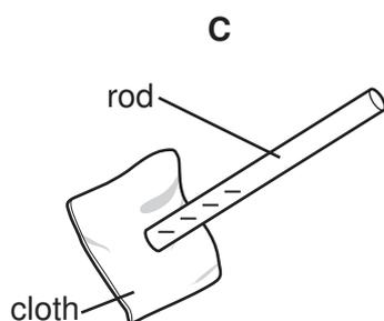
electrons move from the cloth onto the rod
